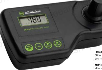
Turbidity is a measure of the clarity of a sample. For potable water applications turbidity is a good indicator of water quality. Turbidity Measurement is achieved by
